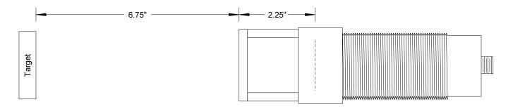
6. Calculate the voltage for the far distance. Add 2.25" to the measured distance and then multiply by the volts per inch. Adjust P2 for the calculated voltage.
