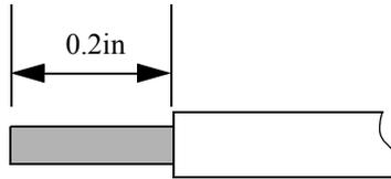
2. Twist the bare wire to fit the terminal hole.
