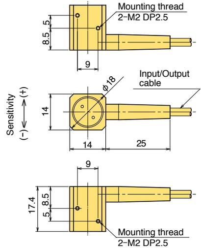
The ARF-A acceleration transducer is used to measure the acceleration of structures subject to vibration such as machinery, vehicles, ships, civil engineering structures, buildings, and so forth. It is small and lightweight and can make measurement on the DC level.
