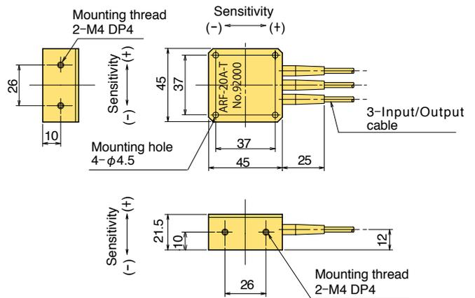
The ARF-A-T acceleration transducer measures acceleration in three directions (X, Y and Z) simultaneously. It is small and lightweight and can make high-accuracy measurement with the least interference.
